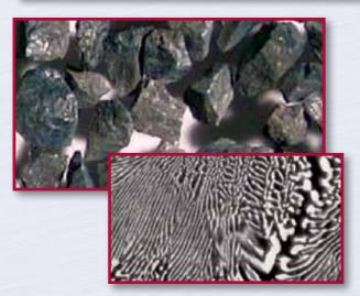
Typical structure of the NorZon Plus grain which has better fracture toughness enabling more controlled fracture behaviour compared with aluminum oxide grain during rapid metal removal.
