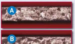
New generation Norton Quantum (A) retains significantly more grain on the edge of a cut wheel compared to high performance Competitor wheels (B).
